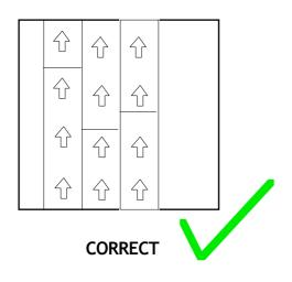
(X) Each roll of Neoflex<sup> $\mathbb{M}$ </sup> is labelled on the underside advising the direction of rolling and which face of the roll is to be placed down on to to sub-floor. Please follow these instructions carefully to avoid potential installation problems.
