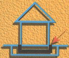
Vibration Insulation of Foundations
