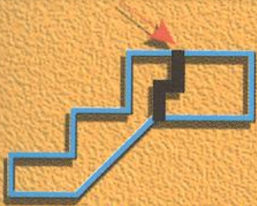
Vibration Insulation of Stairs to Floor
